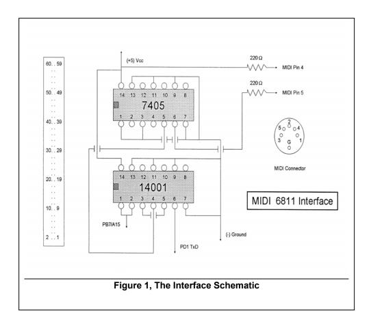
(2) The MIDI standard requires an electrical current of a certain rating to transmit information. Our power supply is 5 volts. We will be using two 220 $\Omega$  resisters in a series, and all MIDI receivers add another 220 $\Omega$  for a total of 660  $\Omega$ . Also, the two gates we use have enough resistance to bring our circuit's total impedance to about 1,000  $\Omega$ .
